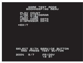
Use the SERVICE Button to move the cursor to the desired test item. Press the TEST Button to enter the selected item. After selecting an item, read the explanations below  $[(A) \sim (E)]$ regarding operation.
