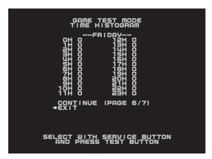
Select CONTINUE with the SERVICE Button and press the TEST Button to advance to the next screen.
