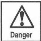
When removing the attachment screws of the monitor door, do not carelessly touch the back of the CRT monitor. There is danger of damaging the cone or receiving a severe electric shock.
