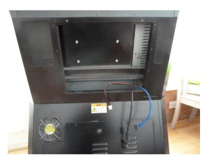
Turn the cab around and take hold of the sides of the monitor frame, lift it out and put it somewhere safe (where you're not going to knock it over).
