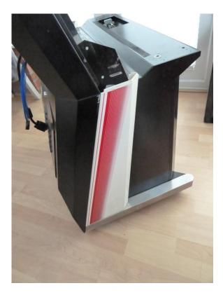
Unlock the rear lower panel and if fitted remove the 3 screws securing it in place (if you have no key - you can remove the nut from the lock from the front of the cab. Remove the PCB shelf.
