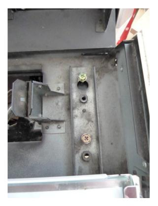
Remove the front one of each set and loosen the rear one - push the panel towards the screen slightly and you can lift the whole control panel assembly off.
