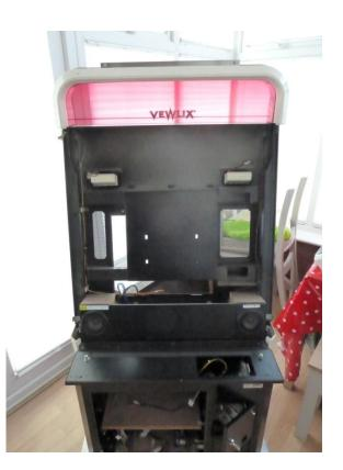
Remove 2 long screws holding these brackets in place - note which way they are mounted - repeat for the other side.
