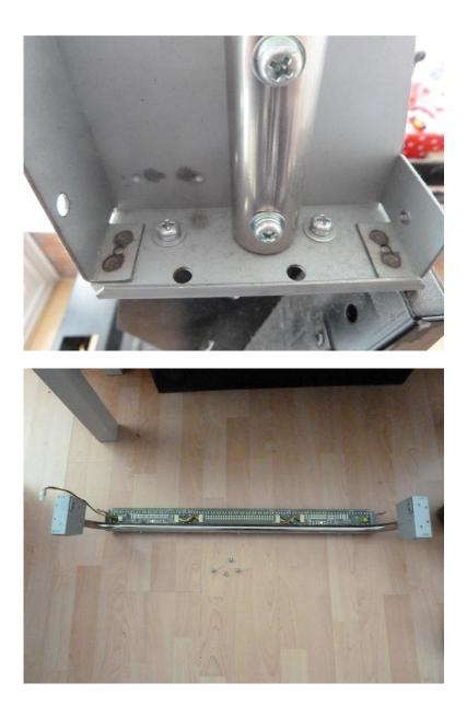
Inspect the top of the cab, there are 3 screws holding a piece of metal that curves around to the front - remove the screws and metal plate.
