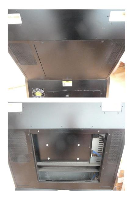
Disconnect the cables from the right-hand side of the screen (Power, Remote, DVI (Optional), VGA). Then undo the 4 bolts.
