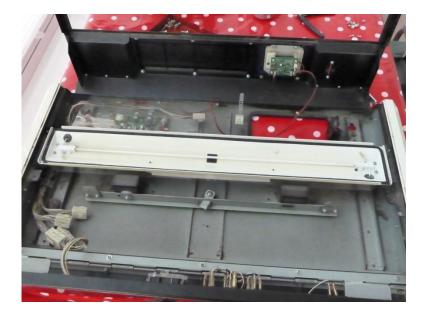
Remove the two screws at both ends on the light strip and it can be removed. NB : some models won't have a light installed – you can fit an LED strip and power it from the 2-pin cable.
