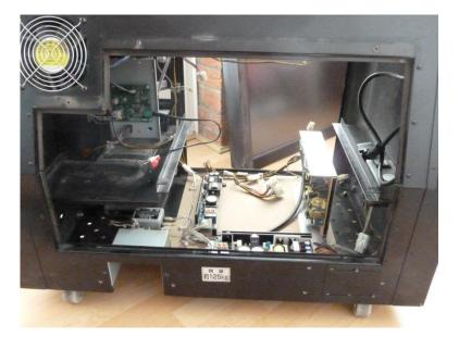
On the side panels there are 5 screws, 2 near the bottom, 2 in the middle and one higher up - these hold the lower side trim in place remove all 10 screws and the side panels lift off.
