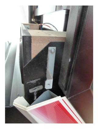
Remove 3 screws holding the long metal plate that runs along the bottom of the speaker unit and remove the metal plate - mine was stuck down with spilt liquid and arcade filth.
