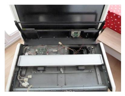
Disconnect cables for IO PCB and light (if fitted) that go through hole in right corner and tuck then into the base.
