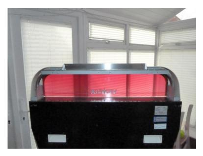
Remove the 2 black screws on the rear that line up with the silver strip at the top of the plastic trim - this releases the metal side trim, remove it and put to one side. If you have a C, F, Diamond there is a 2-pin connector inside the left trim panel, disconnect it (12VDC supply to LED strip in marquee).
