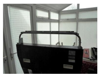
There are 2 screws at each end - undo them and the hoop will lift off (assuming you disconnected the power cable earlier).
