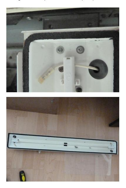
Remove wingnut, unclip cable ties and unbolt earth connection and the JVS/Fastio PCB and loom can be removed.
