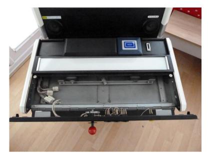
Remove the two large screws at the edges, hinge rear section open.
